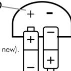
Ensure the batteries are installed correctly. A light to the left of the power button will flash any time a button is pressed. If it does not, reinstall the batteries correctly or check the condition of the batteries.
